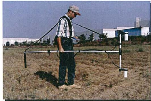
Geometrics G858 Cesium Magnetic Gradiometer
